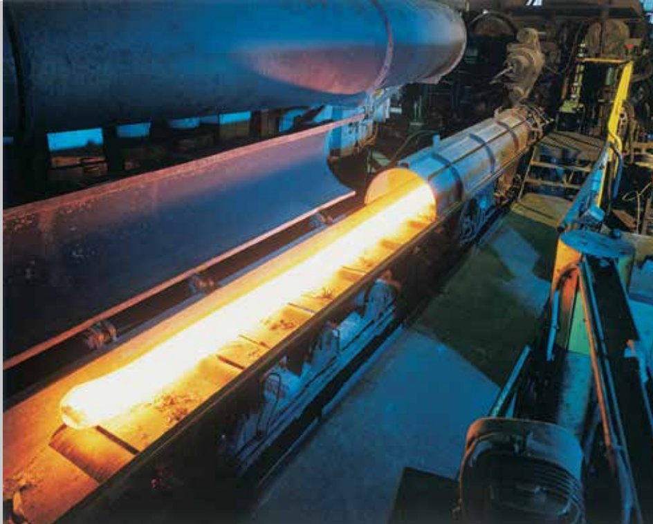
Run-out of the profile bar after extruding through a forming die.
